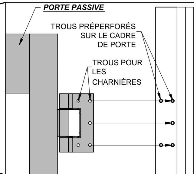
**!** POUR QUE LA PORTE OUVRE ET FERME BIEN, IL EST IMPORTANT D'INSÉRER LES VIS DANS LES TROUS PRÉPERFORÉS DU CADRE DE LA PORTE.
