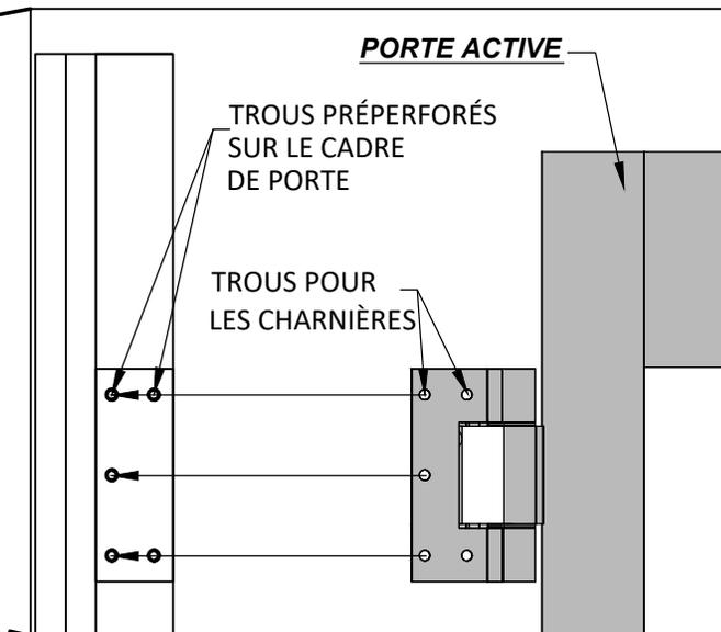
**!** POUR QUE LA PORTE OUVRE ET FERME BIEN, IL EST IMPORTANT D'INSÉRER LES VIS DANS LES TROUS PRÉPERFORÉS DU CADRE DE LA PORTE.
