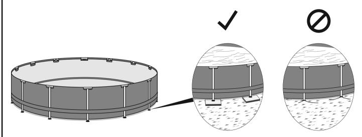
Do not assemble with pool legs on soft lawn. If you must assemble the pool on a soft surface, timber boards (not included) must be placed under the feet of the vertical support rods for even weight distribution. The timber board must meet two conditions:
