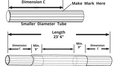
Insert smaller diameter tubes into the large diameter tube, up to the Dimension C mark, as shown. The total length of the tubes should be approximately equal to the corresponding value in Column B. See example on reverse.
