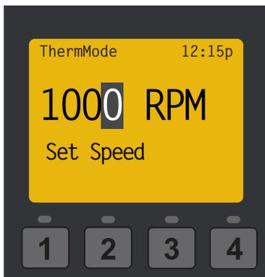
Setting the Thermal Mode Pump Speed
