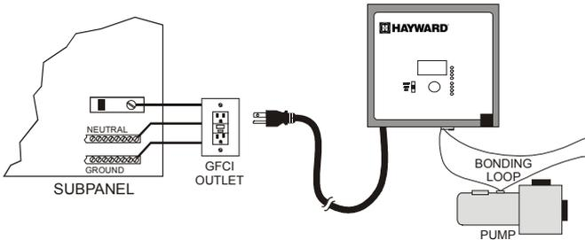
**Bonding:** Lugs used for bonding are attached to the bottom of the Aqua Rite enclosure. Connect to the pool bonding system using minimum 6AWG copper wire.
