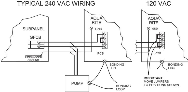
**AQR15XLCUL, AQR9CXLCUL, AQR3XLCUL** - These models are designed to use 120 VAC only. The 120 VAC line cord must be plugged into a GFCI receptacle or a receptacle protected by a Class A ground fault interrupter. See diagram below.
