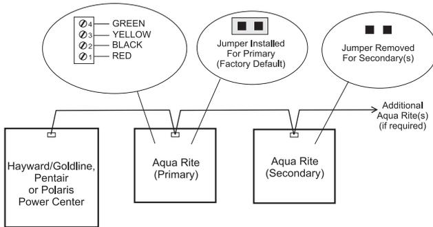
Hayward - Attach wires to proper screw terminals as shown below.
