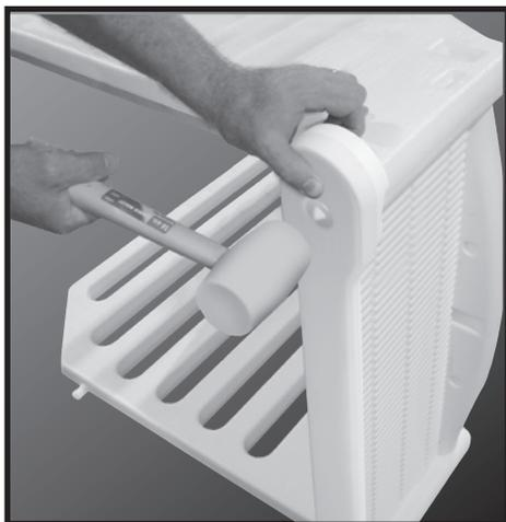
**#7:** Position a stability bar across the front of the step and over each of the round extensions located on the bottom side panels. It will require several hard hits with a rubber mallet to force the stability bar over the extensions. Repeat to install the second stability bar connecting the side panels across the bottom of the step. Stand the step upright.
