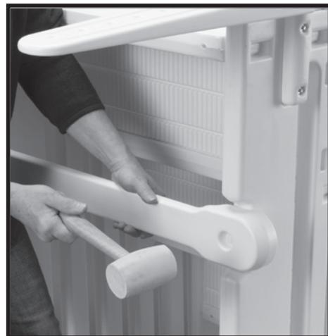
**#7:** Position the final stability bar across the back of the step and over each of the round extensions located on the side panels. It will require several hard hits with a rubber mallet to force the stability bar over the extensions.
