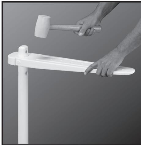
**#3:** If the step is going to be attached to a deck, using the rubber mallet, tap one of the deck connectors onto the bottom (round end) of each of the remaining rail posts. Make sure the flat side of the deck connector is facing the bottom (round end) of the rail post.
