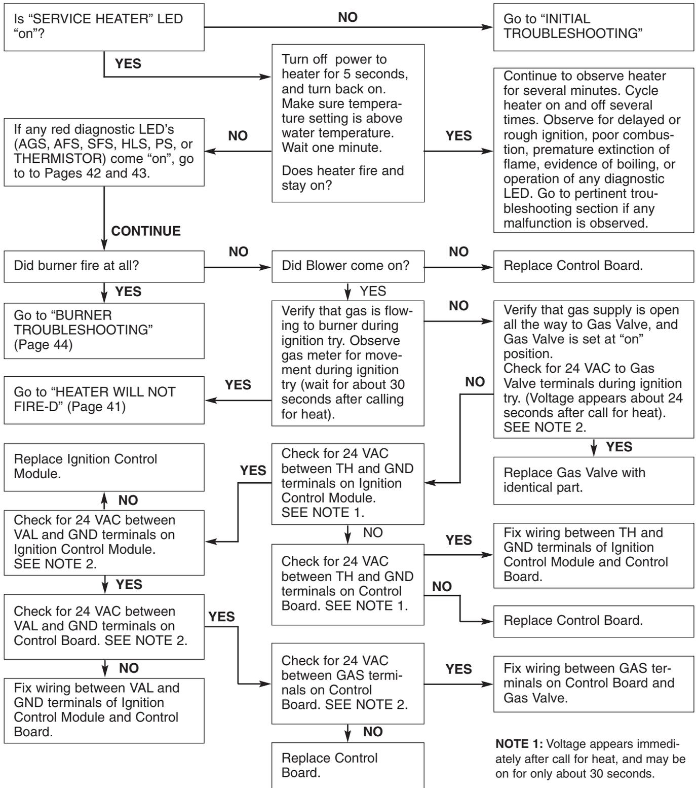
**NOTE 1:** Voltage appears immediately after call for heat, and may be on for only about 30 seconds.
