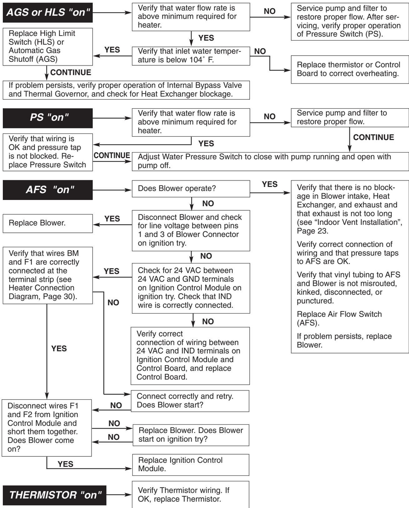
**CAUTION** Do not jumper a safety switch to remedy a failed switch. **NOTE:** ES1 is a spare and should be jumpered.
