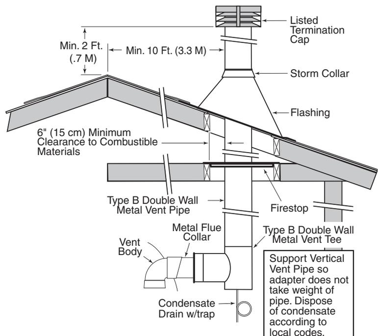
Figure 13. – Typical Metal Vent Pipe Installation - Canada
