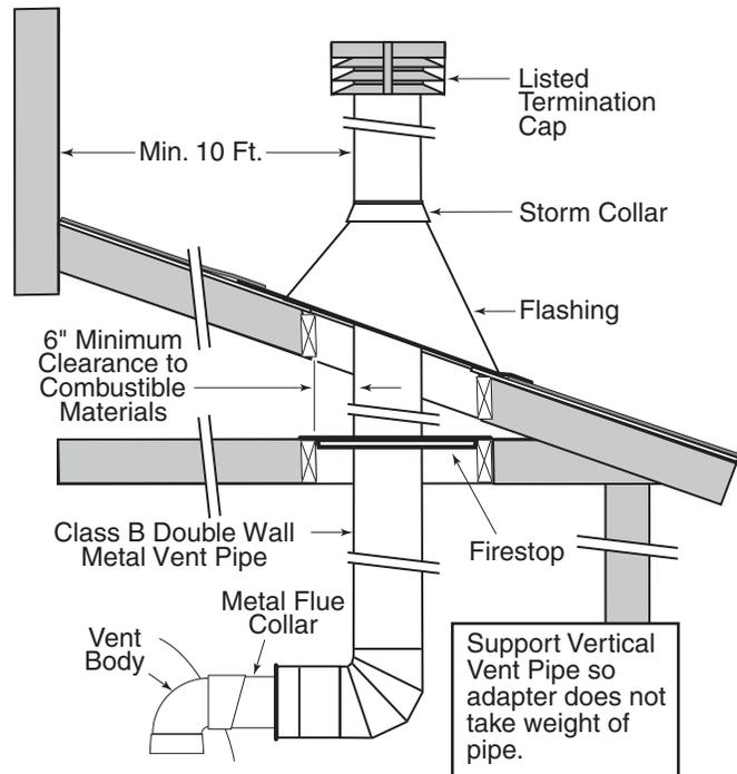
Figure 12. – Typical Metal Vent Pipe Installation - U.S.
