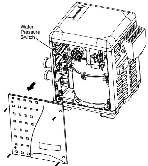
Turn star wheel **clockwise** to raise pressure set point if pressure switch is more than 4 feet (1.2M) below water level
