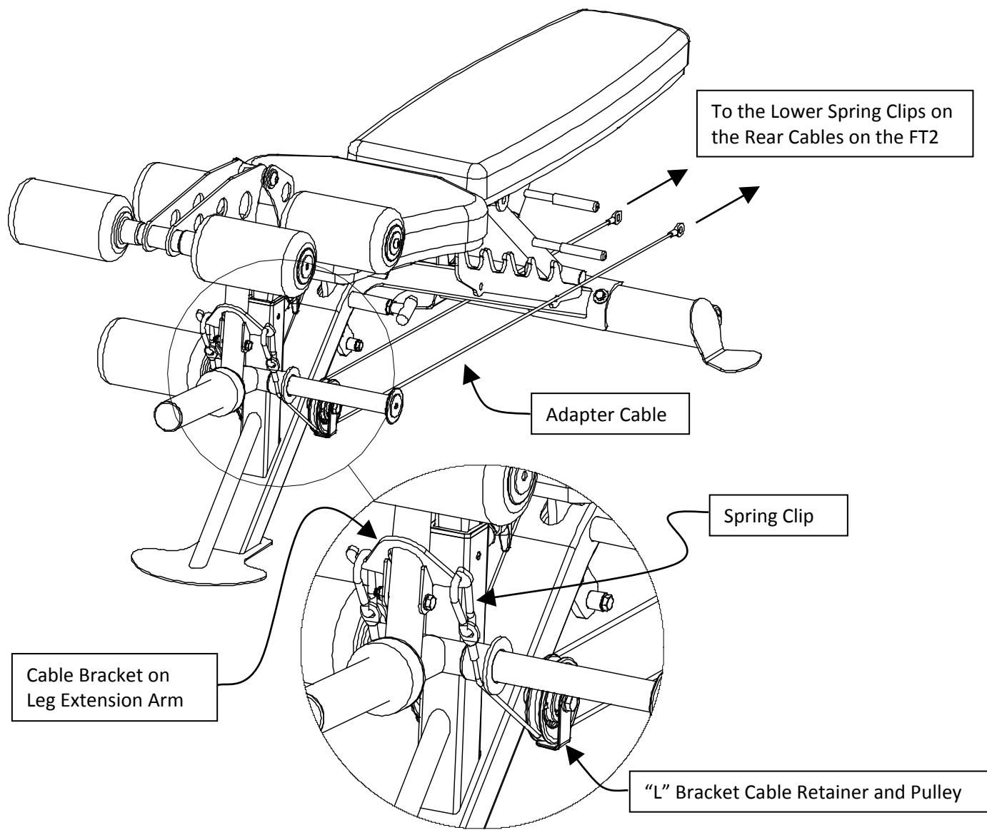
Step 3: Attach one end of the Adapter Cable to the Lower Spring Clip on the Rear Cable of the FT2 machine.
