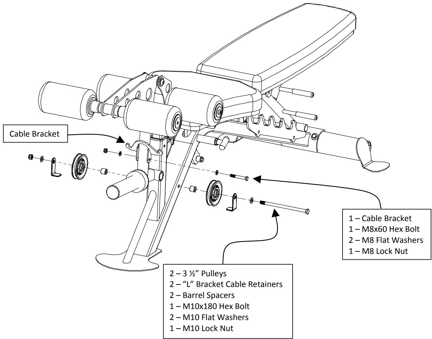
Step 1: Attach two 3 ½" Pulleys, two "L" Bracket Cable Retainers, and two Barrel Spacers to Bench Frame using one M10x180 Hex bolt, two M10 Flat washers, and one M10 Lock Nut.
