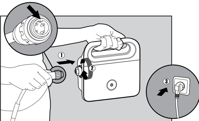
**5.1.3** Attach the floating cable to the power supply by inserting it with the notch on the connector (1), lined up with the groove in the socket on the power supply, and turning clockwise (2). Plug the power supply and leave it in the OFF position (3).
