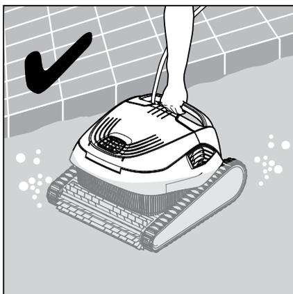
5.4.2 Using the floating cable, bring the Pool Cleaner to the pool's edge. Using the handle, remove the Pool Cleaner from the pool.
