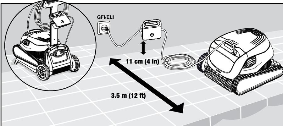
**5.1.1** Position the power supply so that it is approximately in the middle of the long side of the pool at a distance of min 3.5 m (12 ft) from the pool and placed 11 cm (4 in) above ground.
