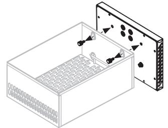
**2** Use four (4) M5x15 screws [j.] to attach the drawer handle to the front panel. Be sure to install handle correctly, with the handle facing down.
