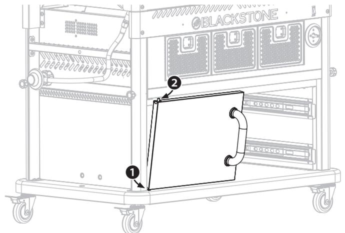
**STEP 15** Use seven (7) M5x10 screws [b.] to attach the cart drawer front panel to the cart drawer body. Repeat this step with the other drawer.
