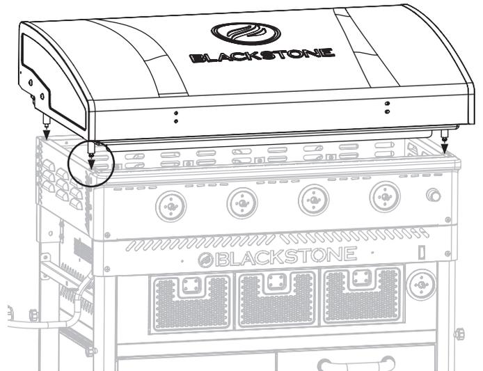
Make sure the front pins are seated in the holes, then push the griddle top back.
