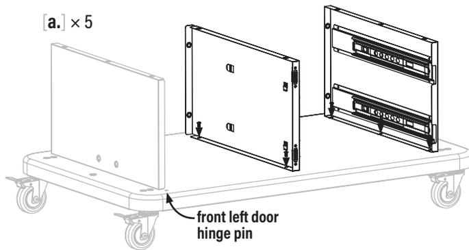
**STEP 04** Use six (6) M5x10 screws [b.] to attach the back cart panel to the left cart panel, middle cart panel and right cart panel.
