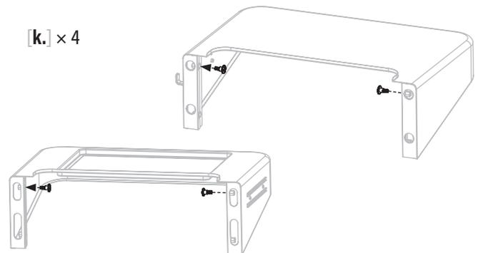
**STEP 25** Slide the left side shelf onto the side shelf brackets. The threaded M6 step bolts will hook and hold the shelf.
