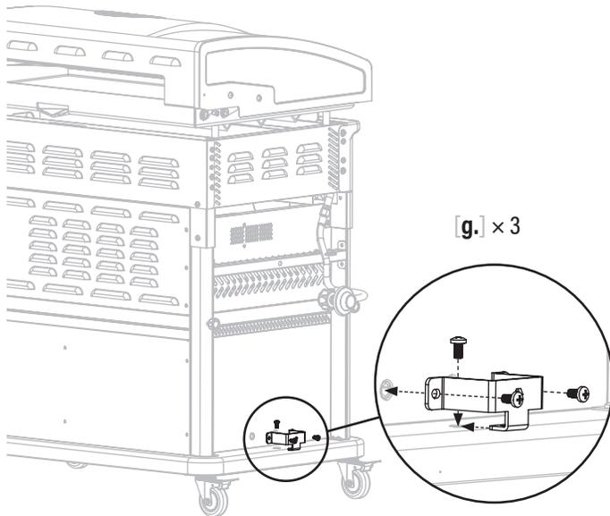
**STEP 20** Use one (1) M6x15 screw [g.] to attach the LPG hook to the left leg assembly. Use one (1) M6x15 screw [g.] to assemble the hose retainer. Use one (1) M6x15 screw [g.] to attach the LPG support to the LPG support bracket.
