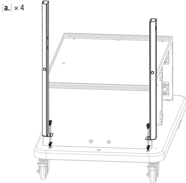
**STEP 07** Use four (4) M6x12 screws [a.] to attach the right-front leg and right-rear leg to the cart base. (**Note:** the front leg is shorter than the rear leg.)
