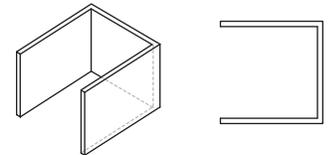
b. Within a partial enclosure that includes an overhead cover and no more than two side-walls. The sidewalls may be parallel, as in a breezeway, or at right angles to each other.
