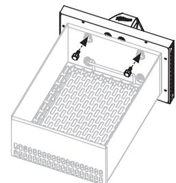
**STEP 27** Place the cutting board onto the right side shelf.
