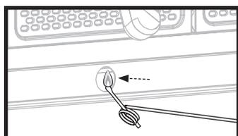
**STEP 04** Push in and turn the control knob to start gas flowing. Ensure burner lights and stays lit.
