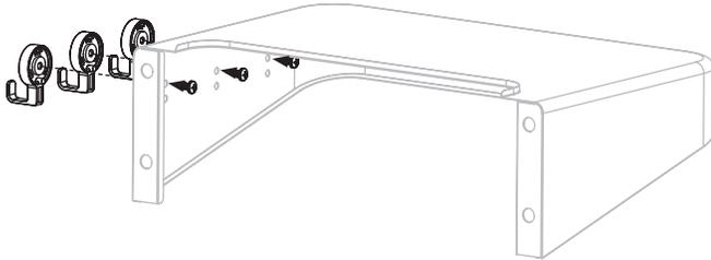
**STEP 24** Thread two (2) short M6 step bolts [k.] into the top holes on the left side shelf. Repeat with the right side shelf.
