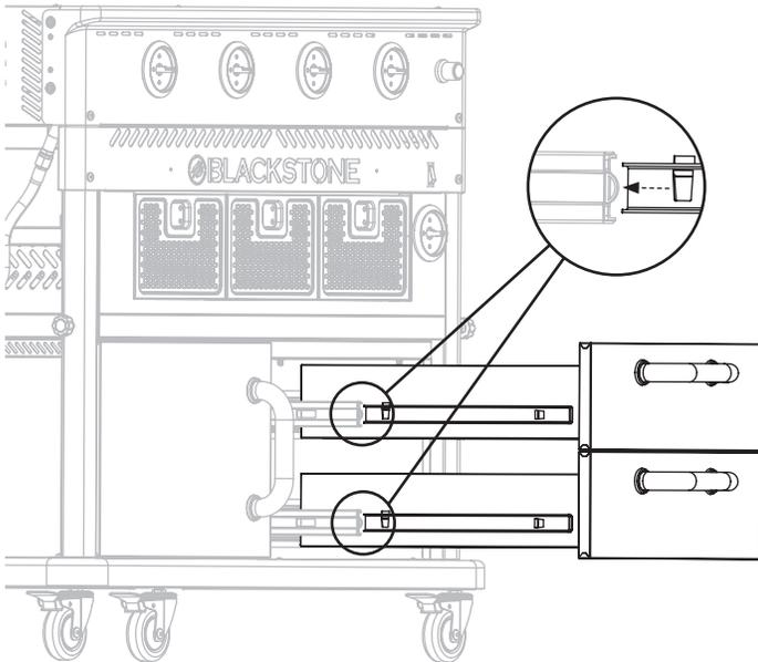
**STEP 18** With the help of another person, place the griddle top and hood on the griddle body by aligning the four (4) pins to the holes of the body.
