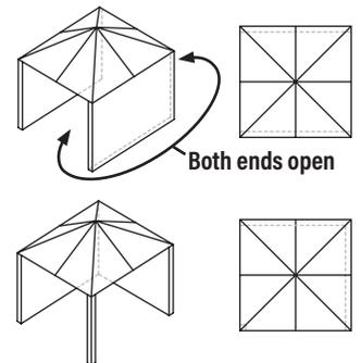
c. Within a partial enclosure that includes an overhead cover and three sidewalls, as long as 30% or more of the horizontal periphery of the enclosure is permanently open.
