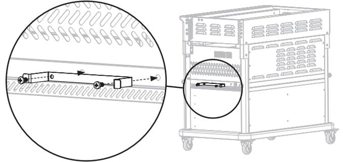
**STEP 12** Use two (2) M5x10 screws [b.] to attach the paper towel holder to the right-front leg.
