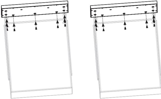
**STEP 16** Use two (2) long step bolts [i.] to attach one (1) cart door/drawer handle and two (2) bezels to the cart drawer front panel. Repeat this step with the other drawer.
