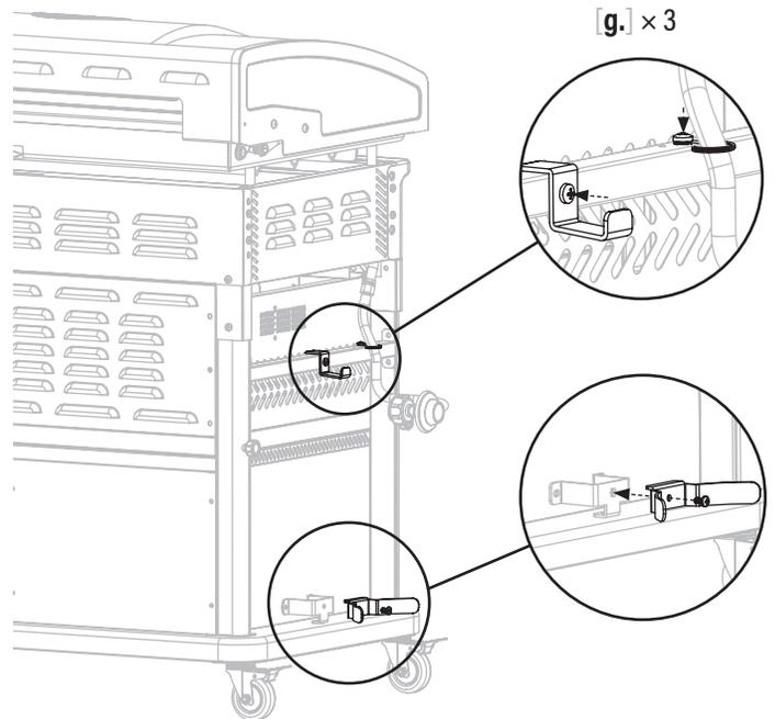
**STEP 21** Slide the hood handle into the two (2) hood handle stand-offs. Use four (4) long M6 shoulder bolts [c.] to attach the handle to the front of the hood.
