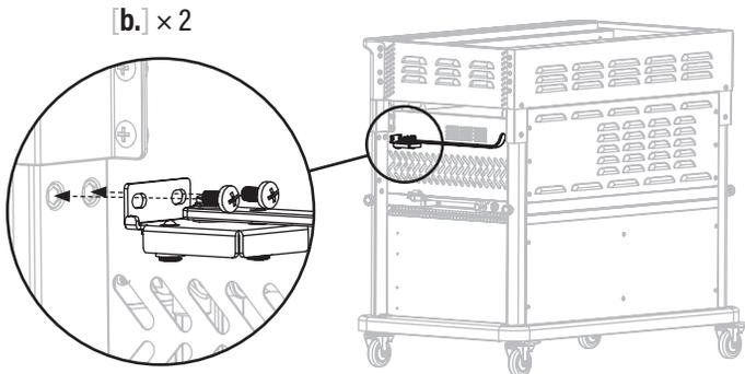
**STEP 13** Use two (2) M6x12 screws [a.] to attach one (1) cart door/drawer handle and two (2) bezels to the cart door.
