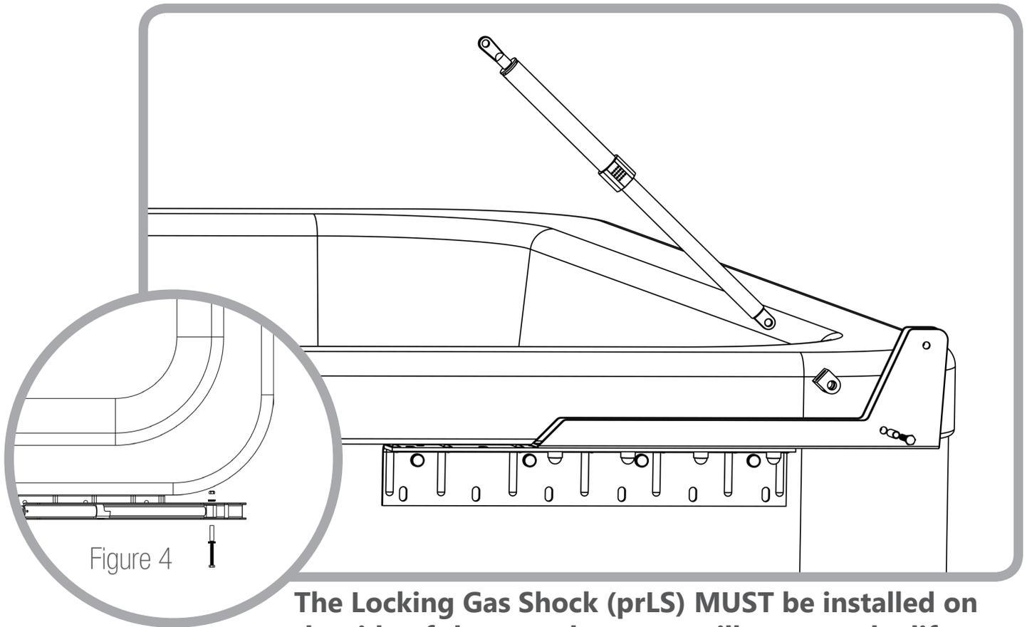
**The Locking Gas Shock (prLS) MUST be installed on the side of the spa where you will operate the lift.**
