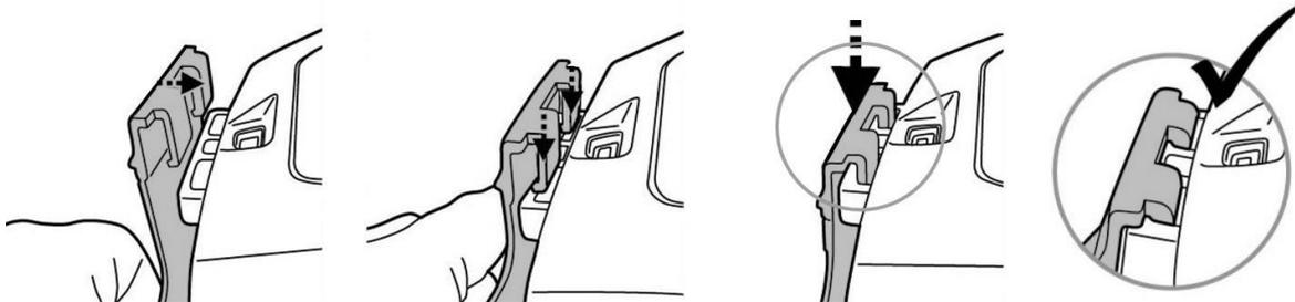
**TIPS:** Press on the two hook ends to remove the rake/brush
