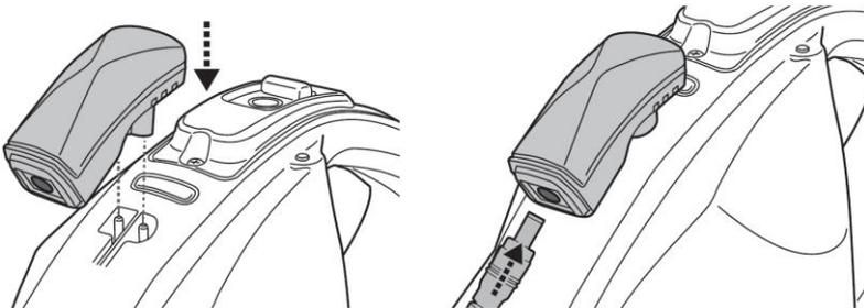
3. Connect the external adaptor to the power source. Once the robot begins charging, the indicator light on the external adaptor will turn red.
