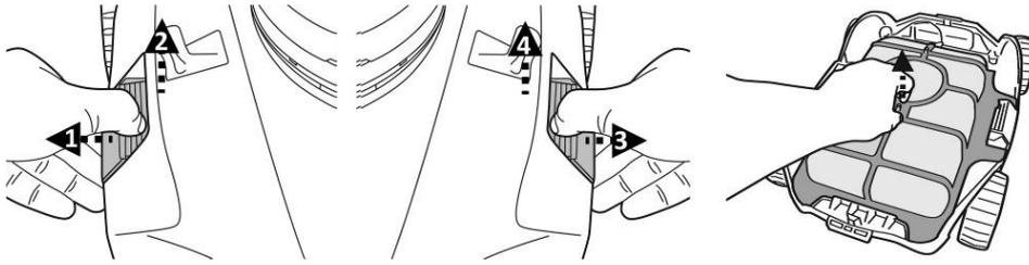
2. Detach the filter cover and remove the debris from the compartment. It is recommended to clean the filter cover net with splashing water. If brushing is deemed necessary, use only a soft brush to clean it carefully and gently to avoid any damage.
