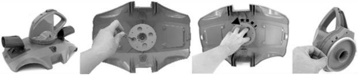
2. Use the screwdriver to unscrew the 4 screws located at the bottom of the head to release the bottom plate first, then unscrew all the screws at the base as shown. Remove the impeller and pry open the base to expose the head inside.
