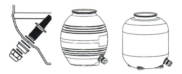
3. Press and turn the sand tank to mount it to sand filter support with correction direction (drain plug is at outside as below pictures).
