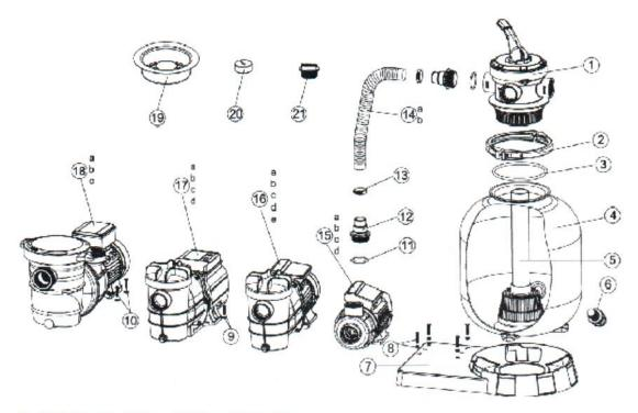
Parts Listing for 14" sand filter with pump
