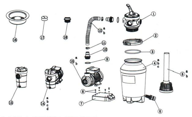
Parts Listing for 10"/12.5"/15" sand filter with pump
