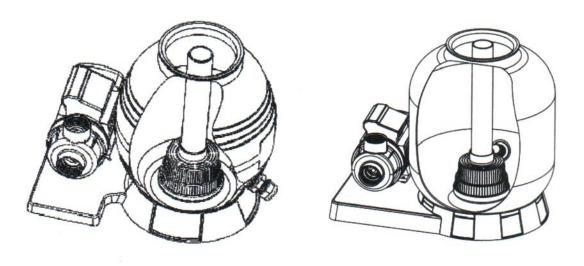
**4**.Insert the tube with the diffuser body inside the tank as above picture, then place the funnel on the tank's mouth and pour the quartz sand into the tank (12 inch sand filter needs about 19kg sands to fill into the tank,14 inch sand filer needs about 27kg sands to fill into the tank).
