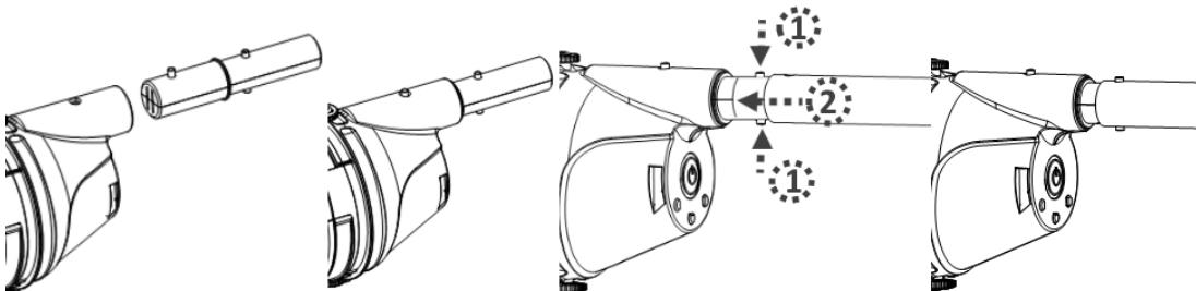
To release the telescopic pole, press down on the two side pins simultaneously and pull out the pole.
