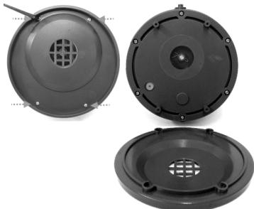
3. Unfasten 6 screws and detach the cover to expose the PCBA, motor assembly, and battery pack.
