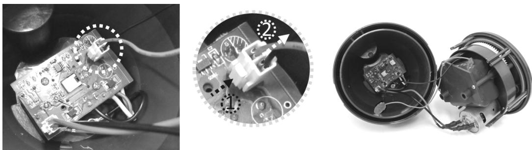
4. Unfasten the 3 screws to release the battery compartment cover. Remove battery pack from the compartment.
