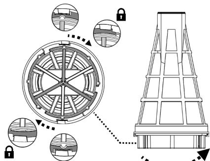
6. To re-position the transparent canister (with filter cone inside) onto the rear body, make sure the locking knob on each side is turned to the unlocked position. Align the raised arches on both sides of the transparent canister with the locking knobs and turn each knob clockwise until it points towards the red marking to secure the assembly.
