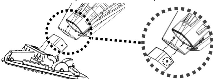
NOTE: To replace the brushes on the suction head, lift the end and pull it out to make space for a new one.
