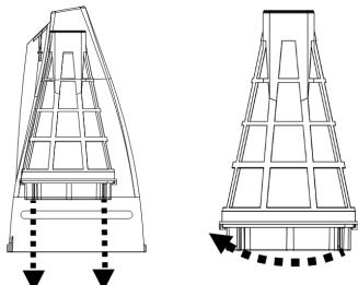
4. Rinse the transparent case and clean out the debris inside the filter cone. It is recommended to clean the filter cone's net with splashing water. If brushing is deemed necessary, use only a soft brush to clean it carefully and gently. DO NOT apply any pressure to the net.
