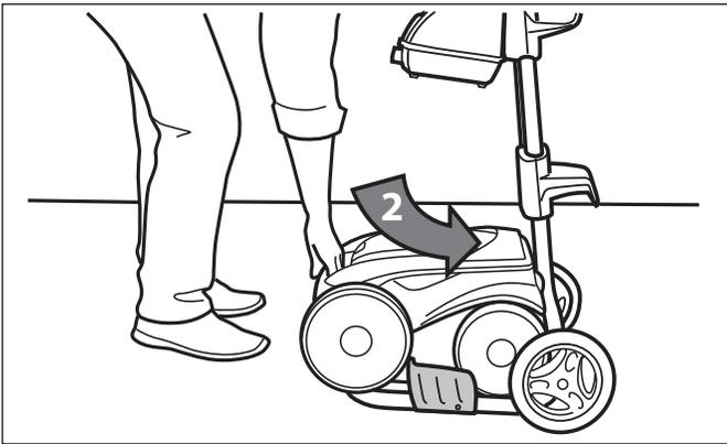
**Figure 29. Roll Cleaner onto Place on the Caddy**
